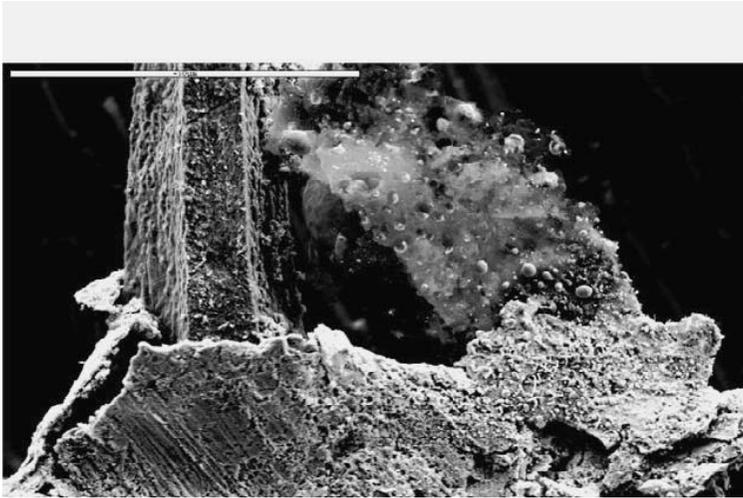
Fig. 3. The same particles as in Figure 2 after storage at ambient for 11 days. The spherical particles and the surrounding matrix in the upper right quadrant were analyzed using EDS.
