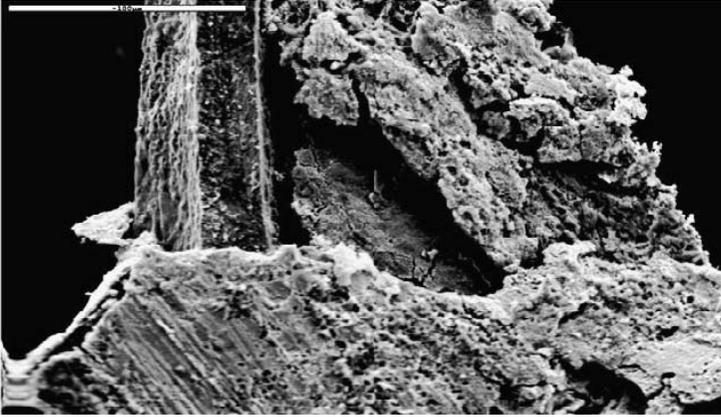
Fig. 2. Floating particles were collected from the electrolyte surface after electrolysis.
