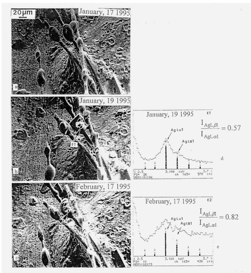
Fig. 1. (a–c) Changes in morphology of fibers which formed on a Pd cathode during electrolysis. These changes occurred during storage at room temperature. (d, e) EDS spectra showing changes in composition which were detected at spot E1 on January 19, 1995 and at spot E2 on February 17, 1995.
