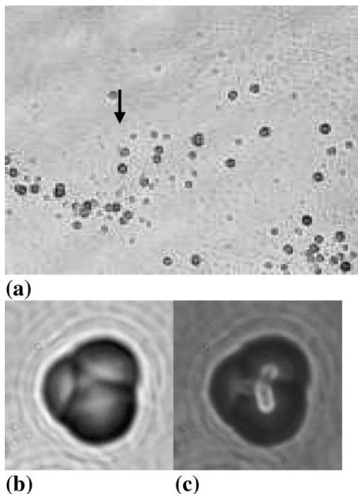
Fig. 3. (a)  $\times 200$  magnification of a cloudy area observed where the Ag/Pd cathode was in contact with the CR-39 detector during an external magnetic field experiment. Arrow indicates a “triple” pit. Images of the triple pit obtained at  $\times 1000$  magnification where (b) the focus is on the surface of the CR-39 detector and (c) the image is an overlay of two images taken at two different focal lengths (top and bottom of pit).
