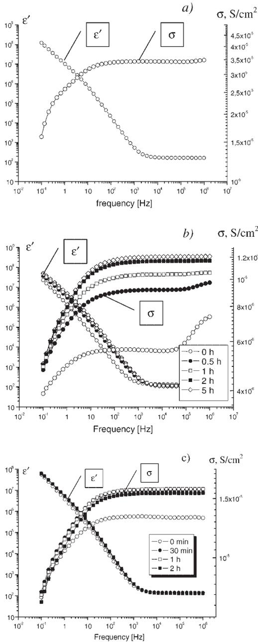
Fig. 1. Dielectric permittivity  $\epsilon'$  and conductivity  $\sigma$  of a water versus the frequency: (a) initial non-activated distilled water at 20°C; (b) the same distilled water activated for 30 min and stored at a temperature of 20°C; (c) the same water activated for 30 min and stored at a temperature of 40°C.
