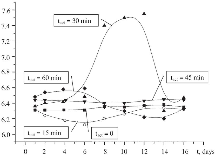
Fig. 3. Influence of the water activation duration on pH depending of the time of its storage at a temperature of 20°C.
