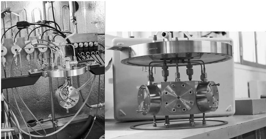
Fig. 1. (Left) Single electrolytic cell and its wiring inside the thermostatic box; (right) multiple cells device.
