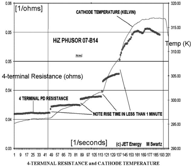
Fig. 2. Pd resistance and temperature of a Type "B" Phusor LANR device.
