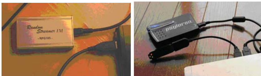
Figure 2. Two RNG devices, Random Streamer (Rpg 105 and Rpg102) and Psyleron (REG-1), are shown connected to the PC.
